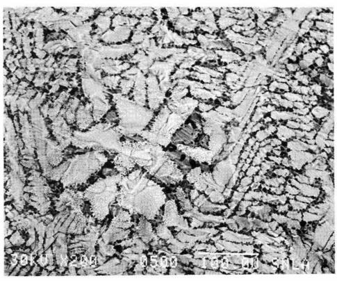
USING a new backscattering electron detector, Sandia scientists in Dept. 5820 have been able to make a direct correlation of glass ceramic fracture surface features (top) with the underlying microstructure.
